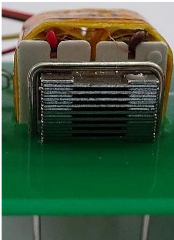
Now cut the transformer wires to length and strip and tin them. Connect the wires to the PCB as shown in the picture below:
