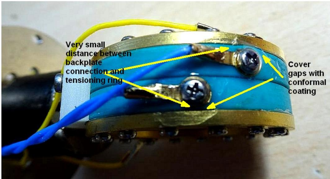
It is a good idea to mark which wire is coming from the front membrane and which wire is coming from the rear membrane. The backplate connection(s) usually have a different wire color, so the function of this wire is clear.
