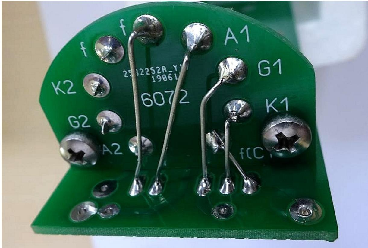
f(CT) of the tube PCB connects to CT on the main PCB
