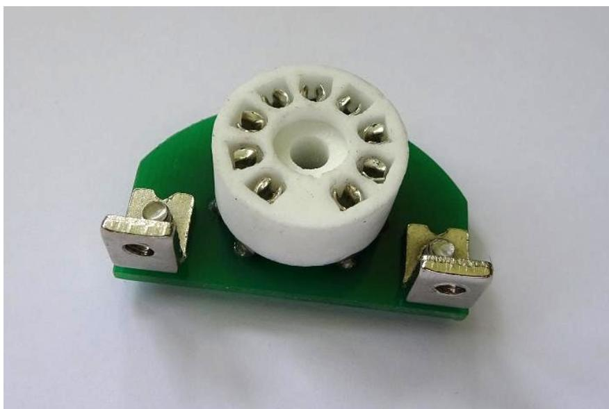
Now mount the small tube PCB to the main PCB with two M3 screws, as shown below. We have to make a couple of connections now...
