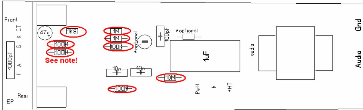
Now place and solder the two 10 nF (0.01) /630V capacitors, the 100pF capacitor, the 1000 pF styroflex capacitor and the 47 µF electrolytic capacitor. Take care of the orientation of the electrolytic capacitor, the '-' side should be at the corner of the PCB, close to the bigger 3 mm. hole. Finally we place and solder the yellow 1 µF/250 V capacitor.
